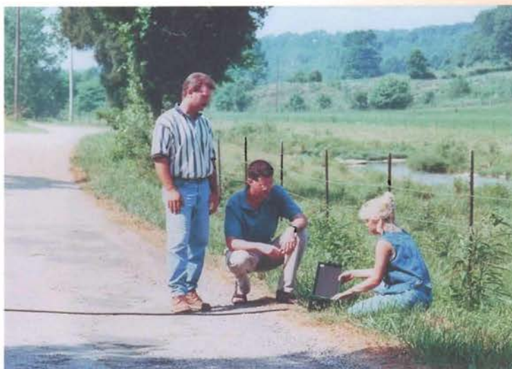
DARIN DUNCAN, HIGHWAY ENGINEER, TOM MAHON, GRADUATE ENGINEER, AND HEATHER BALENTINE, CIVIL ENGINEERING SUMMER INTERN, SET UP A TRAFFIC COUNTER.
